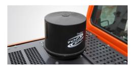
PRE CLEANER The installation of a rotor type pre-cleaner has increased filtering efficiency by 5~10%.
