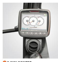
**2** 7-INCH MONITOR The new, user-friendly LCD color monitor provides a clearer rear view and allows full access to machine settings and maintenance data. (Rear view camera is optional.)
