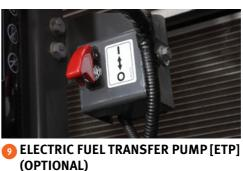
The adoption of pump switch enables easy refueling of the machine after inspection or repair.
