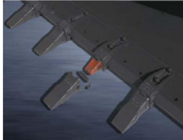
2-Piece Type Tooth(Pin-on+Bolt-on adapter)
