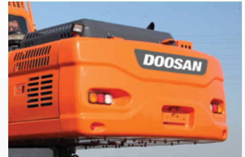
Low center of gravity designed Counter-weight
