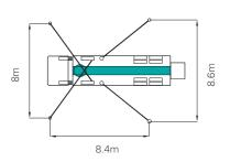
Front outrigger type X(Diagonal) Extension Rear outrigger type Swing-out
