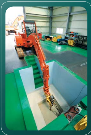
Test unit installed on impact base connected with strain gauge in tool bit and flow and pressure gauge on hoses port of cylinder
